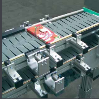
System EL-195 für Transport von Schokolade EL-195 conveying system for chocolate
