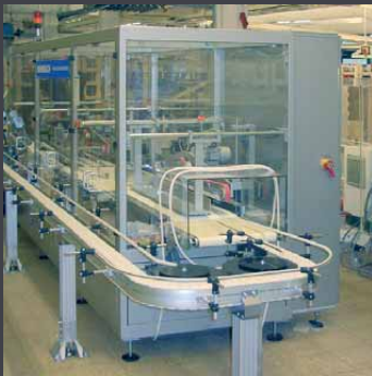
System EL-85 für Transport von Backwaren EL-85 conveying system for bakery goods
